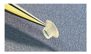
• The front plate is a solid piece of PMMA with a mushroom shape, with an anterior lip (5.0 mm in diameter), and stem (3.35 mm in diameter).
